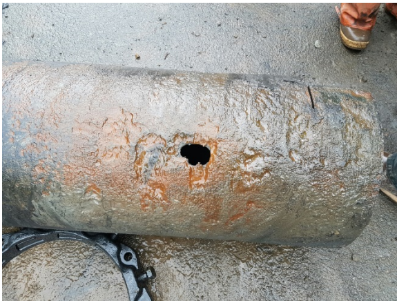
Water main line break and repair near Pt. Lena Loop Road
